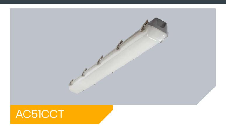
CCT switchable between 3000K, 4000K & 6500K. Tough exterior provides an IP65 and IK08 housing protecting the LED components inside. 304 stainless steel clips for high corrosion resistance and anti-tamper screws for vandal proofing. Unique gear tray slots that allow us to easily integrate third party control gear for your project. Safety tether cable to gear tray enables fast installation. Compression cable gland included in fixings kit. BESA mounting kit available.
