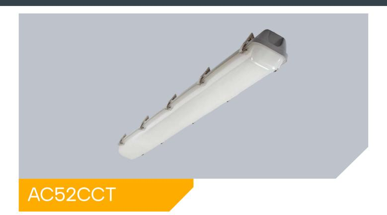
CCT switchable between 3000K, 4000K & 6500K. Tough exterior provides an IP65 and IK08 housing protecting the LED components inside. 304 stainless steel clips for high corrosion resistance and anti-tamper screws for vandal proofing. Unique gear tray slots that allow us to easily integrate third party control gear for your project. Safety tether cable to gear tray enables fast installation. Compression cable gland included in fixings kit. BESA mounting kit available.
