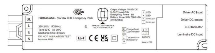
When the self-test system is active(link removed), a functional test is carried out automatically once a week and runs for 30seconds. A full duration test is carried out automatically every 52 weeks. The first full duration test is carried out automatically within the first 4 weeks of being connected to mains supply.
