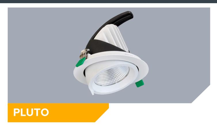
Pluto provides multi-directional wallwash/accent lighting with rotation and angle adjustments. Its adjustable head rotation of  $340^{\circ}$  and tiltable head of  $-18^{\circ}$  to  $+45^{\circ}$  make them perfect for internal sign lighting. The series comes in three sizes and two colour temperatures, with dimmable and emergency options.
