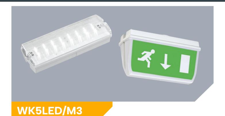
**WK5**LED bulkhead utilises an IP65 rated polycarbonate base and fresnel lens housing 16 high output white LEDs and constant current maintained drive circuit.
